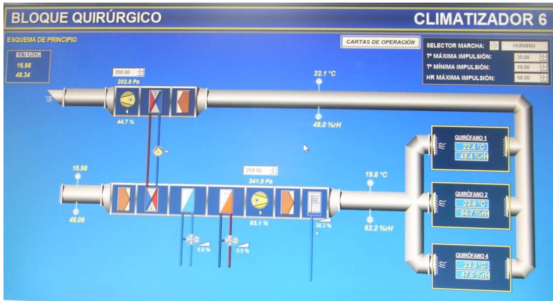
Figure 15. Screenshot from the BMS interface where one of the AHUs (with energy recovery) installed in Areilza (Surgical Block) building can be seen in detail
