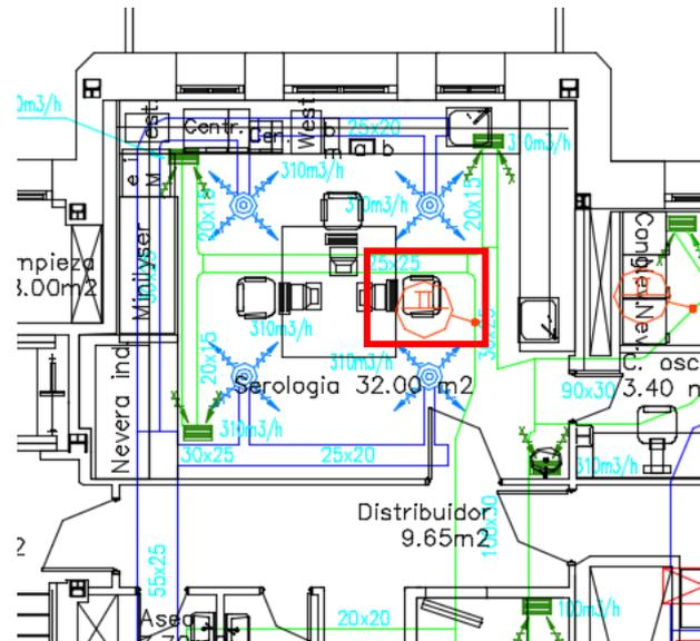
Figure 3. Sensor located on the return duct from a room (Serologia)
