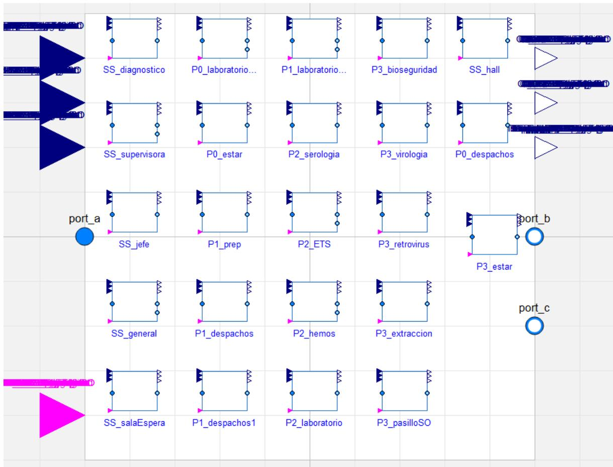
Figure 80. Gurtubay AHU SO zoning Modelica model.
