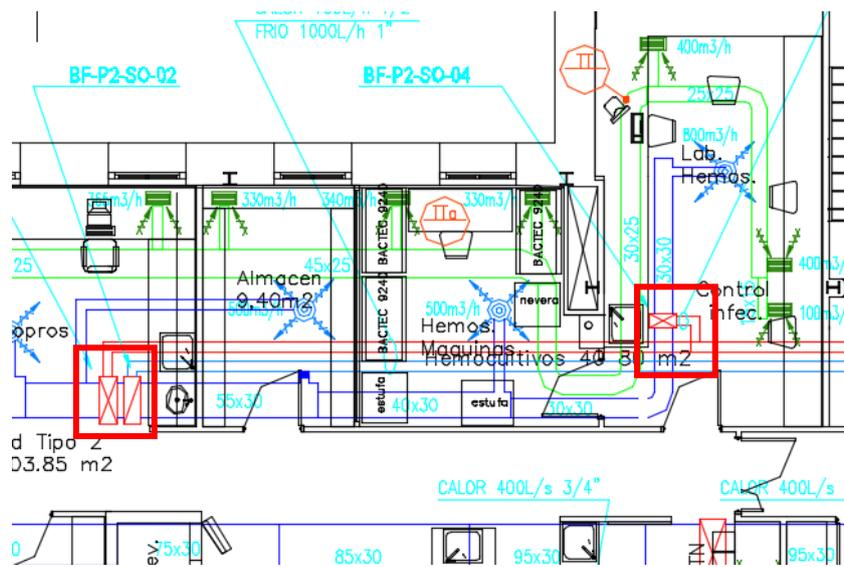
Figure 2. Post heating coils
