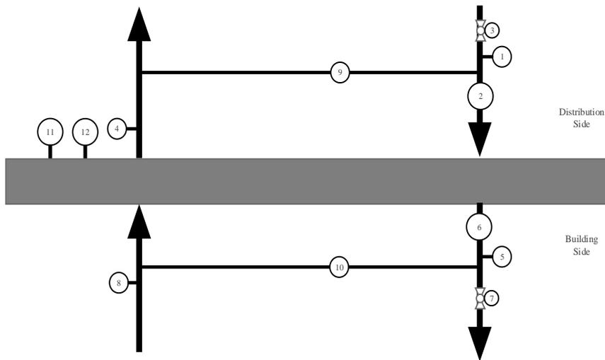
Figure 67. Substation input/output variables location
