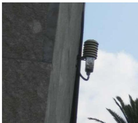
Figure 26. External measurement equipment for air temperature (Francesco Passerini, 2016)
