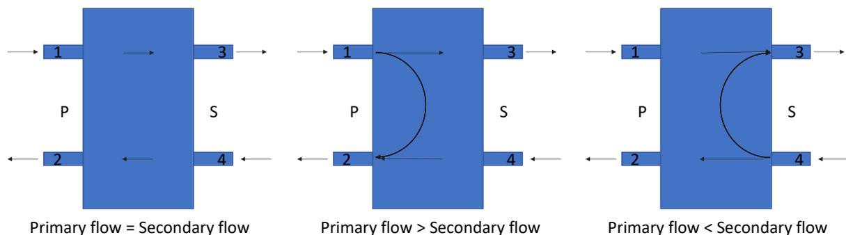
Figure 65. Substation heat transfer according to mass flow rate relations
