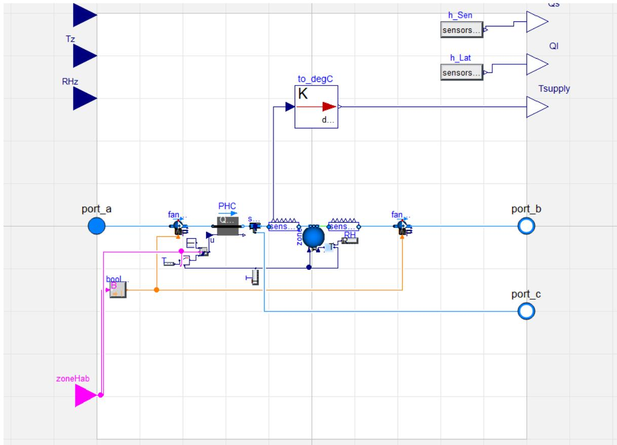
Figure 47. zonePHC\_PCC\_splitSupply Modelica model
