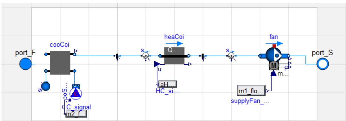
Figure 56. AHU Type 2 Modelica model.
