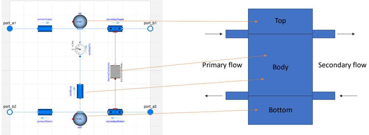
Figure 66. Substation Modelica Model
