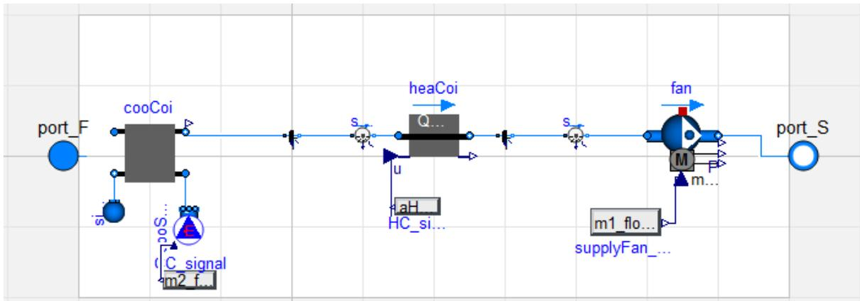
Figure 58. AHU Type 3 Modelica model.
