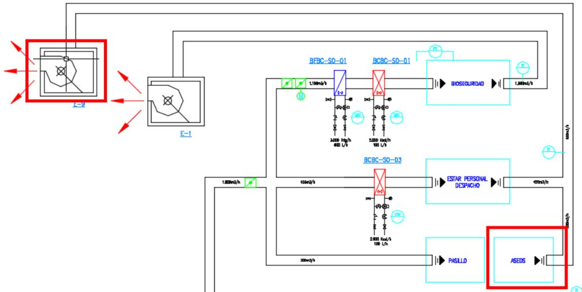
Figure 11. Zone in depression without supply vent
