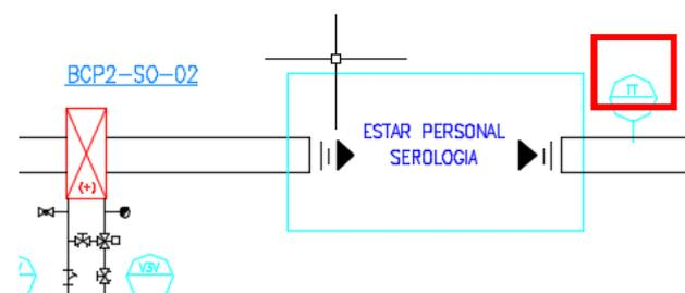
Figure 4. Sensor located on the return duct from a room (Serologia)
