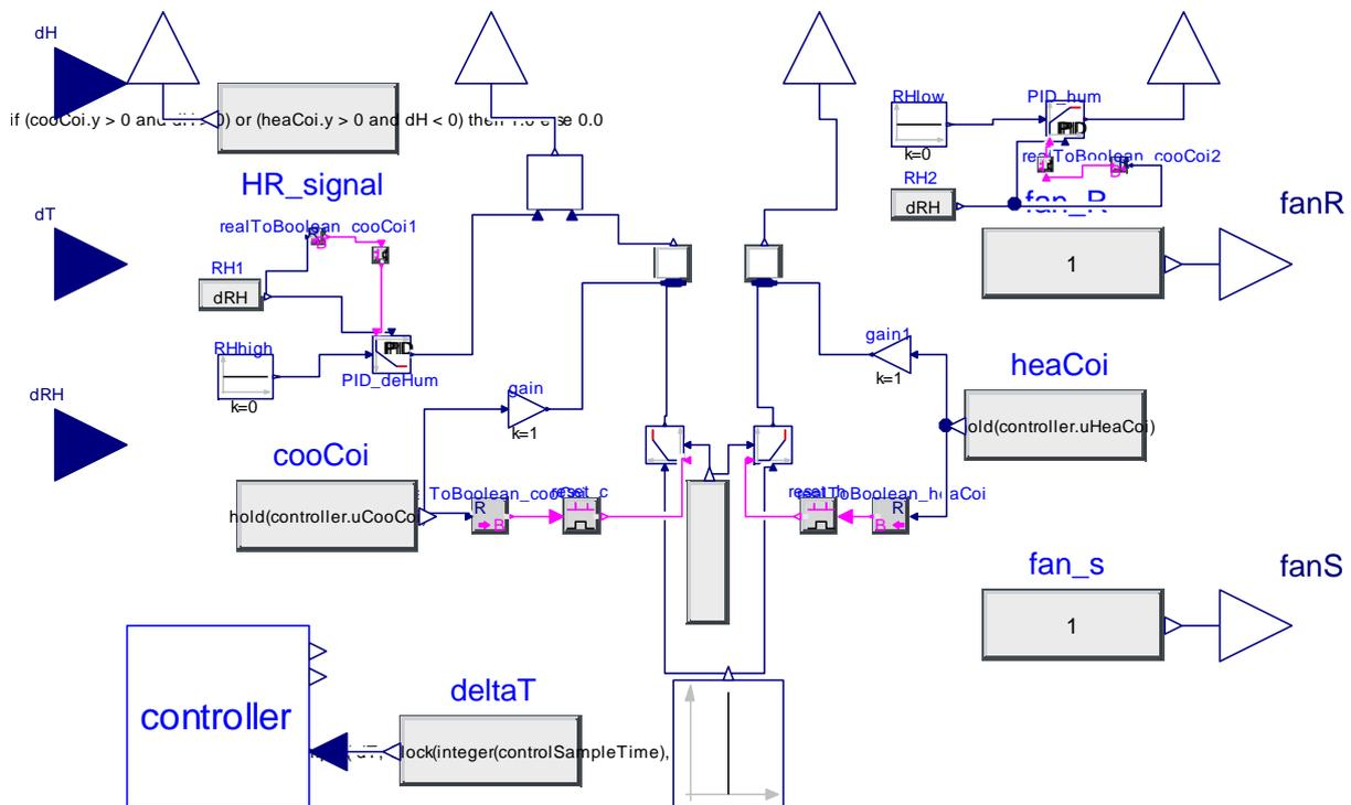
Figure 63. AHU\_controller Dymola representation
