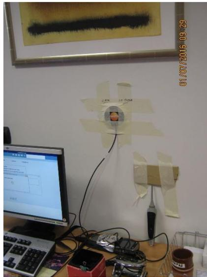
Figure 24. Internal measurement equipment for heat flow rate, surface temperature, and air temperature (Francesco Passerini, 2016)
