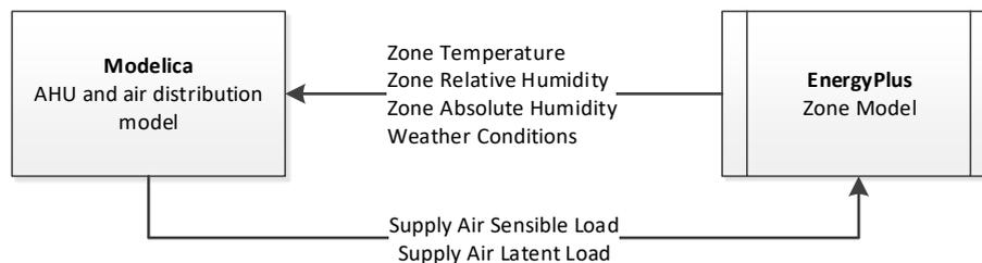
Figure 42. Modelica/EnergyPlus data exchange diagram
