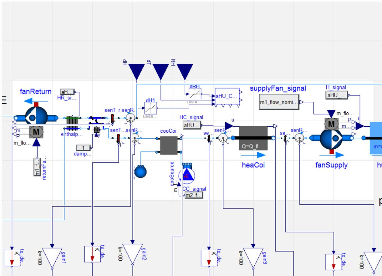
Figure 62. AHU Type 5 Modelica model.
