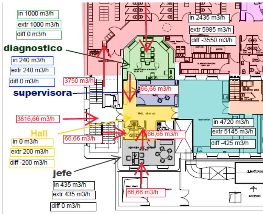
Figure 9. The zone Hall is in depression without supply vent
