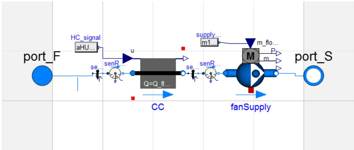
Figure 52. AHU Type 0/Fan coil Modelica model.
