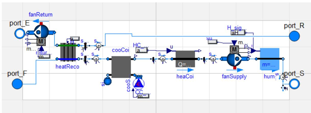
Figure 54. AHU Type 1 Modelica model.
