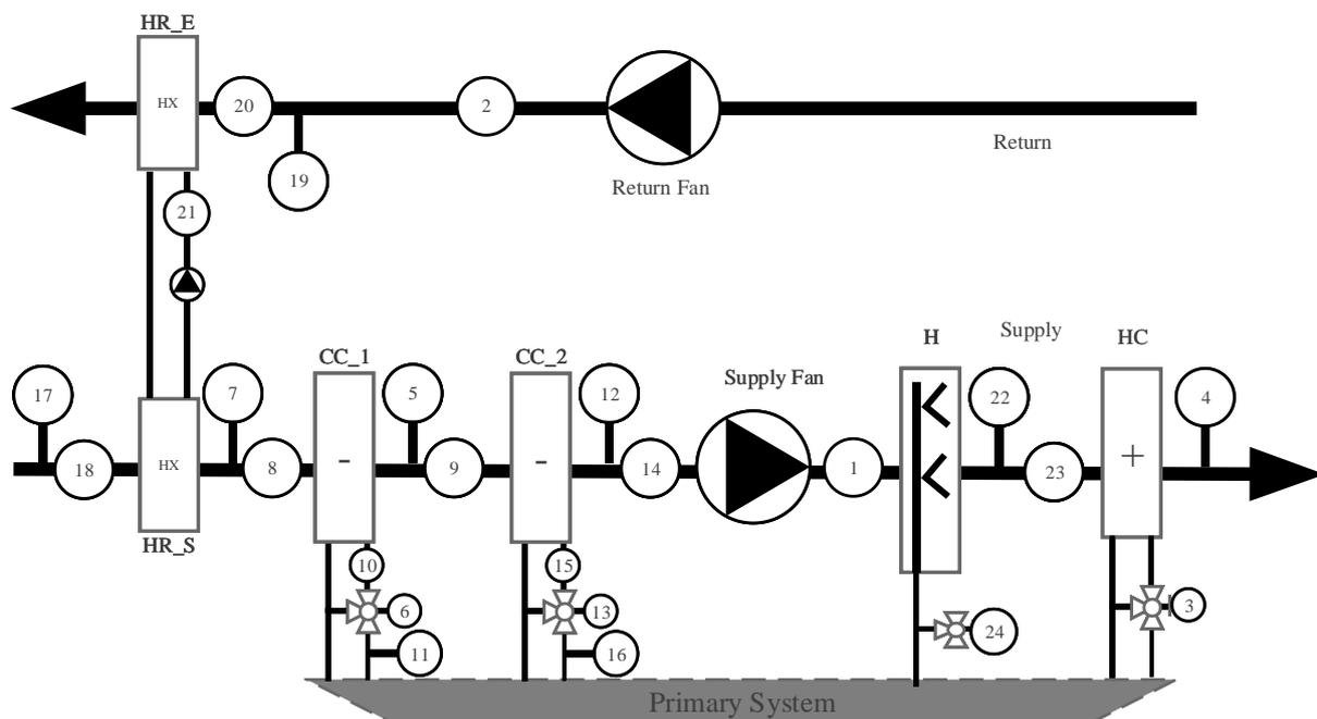
Figure 57. Type 3 schematic.
