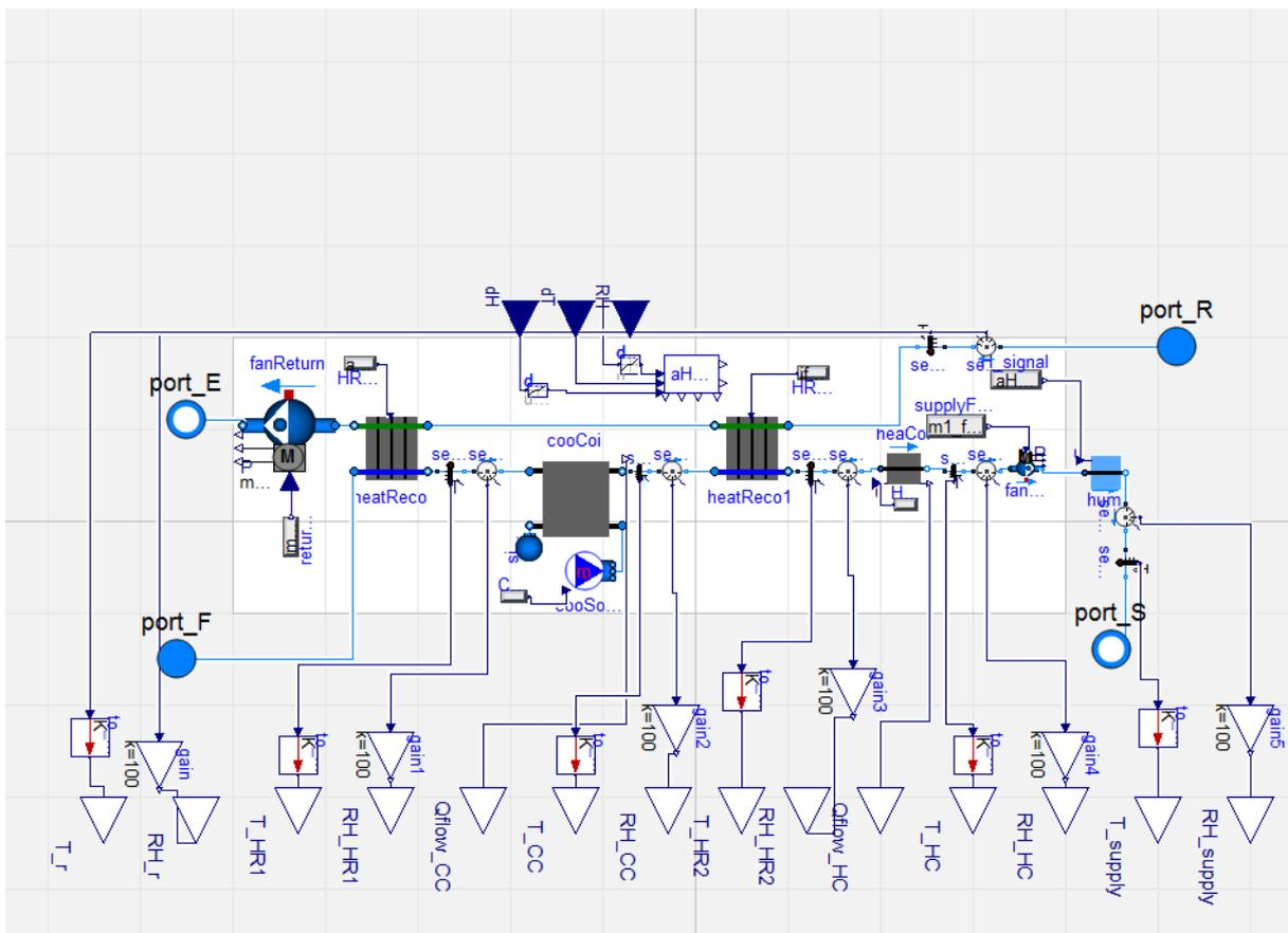
Figure 60. AHU Type 4 Modelica model.
