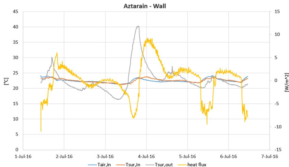
Figure 27. Elaboration of measured data relative to an external wall of Aztarain building (Francesco Passerini, 2016)
