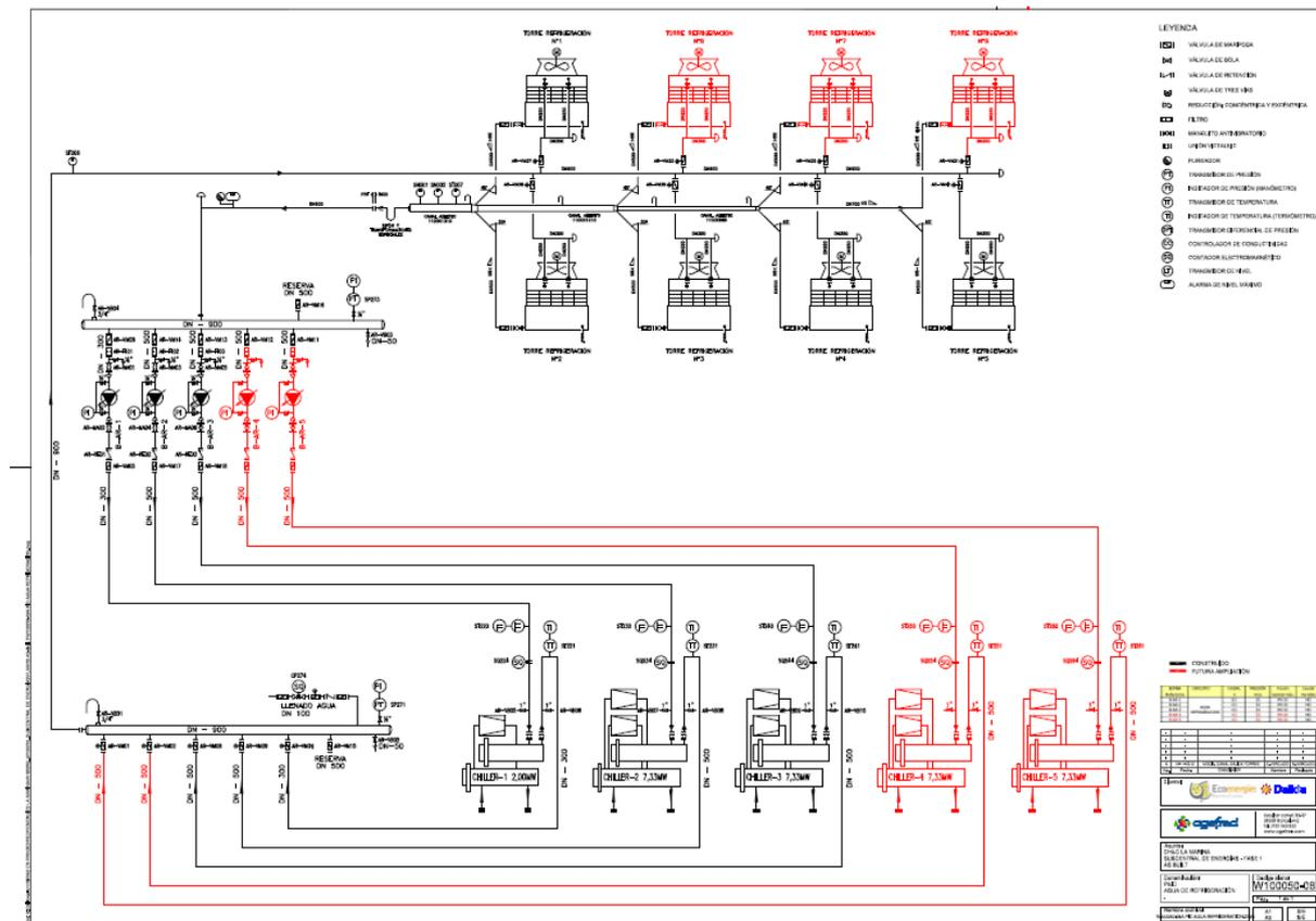
Figure 5. Schematic of the chillers and corresponding cooling towers in La Marina test site.
