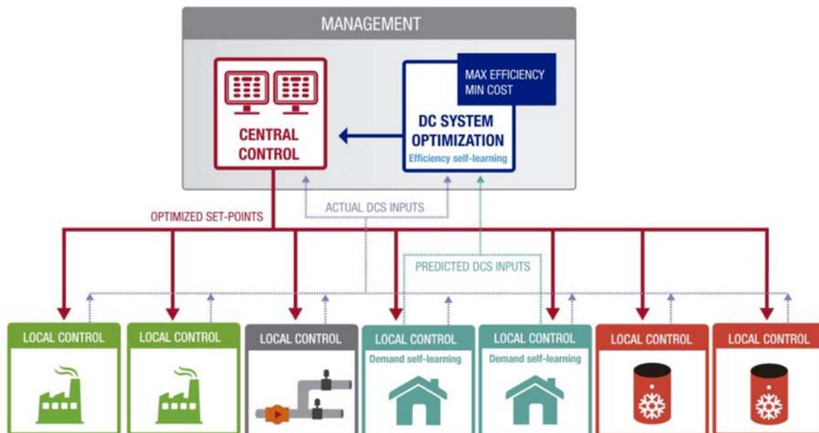
Figure 2: Overview of INDIGO controller hierarchical structure
